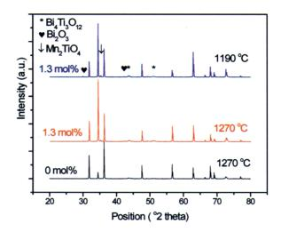
Fig. 1: XRD pattern at different doping level of MnO<sub>2</sub>
