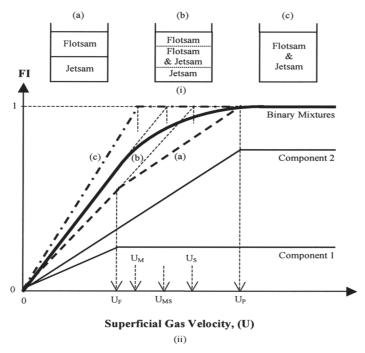
Fig. 1: Relationship between bed pressure drop and gas velocity for fluidization of binary particles system
