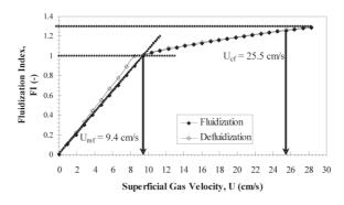
Fig. 4: Fluidization index versus superficial gas velocity for mixture of 85% silica sand and 15% palm pressed fibre
