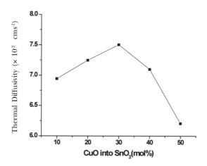
Fig. 4: Thermal diffusivity of SnO<sub>2</sub>-CuO at different composition
