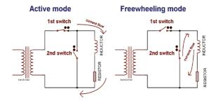
Fig. 2: AC controller operation modes
