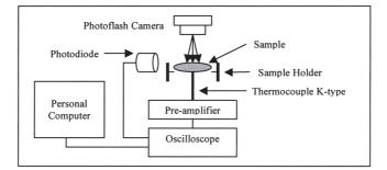
Fig. 1: Schematic diagram of the photoflash technique
