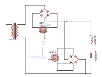
Fig. 1: Circuit diagram of symmetrical PWM AC chopper
