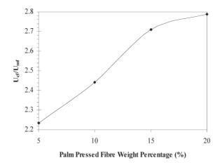
Fig. 7:  $U_{cf}/U_{mf}$  ratio for mixture of silica sand and palm pressed fibre
