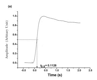
Fig. 3: Thermogram of SC1 sample (thickness, L=0.2354 cm)
