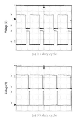
Fig. 4: Triggering signals with variable duty cycles
