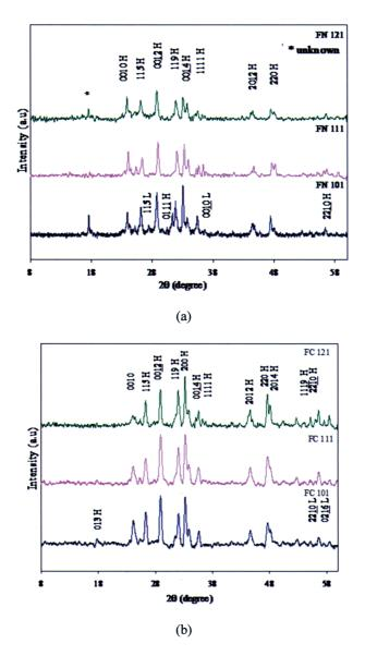
Fig. 2: XRD spectrum for (a)(Bi,Pb)<sub>2</sub>Sr<sub>2</sub>Ca<sub>2</sub>Cu<sub>3</sub>O<sub>10</sub>, 840°C (FN101), 845°C (FN111) and 850°C (FN121) (b)(Bi,Pb)<sub>2</sub>Sr<sub>2</sub>Ca<sub>2</sub>Cu<sub>3</sub>O<sub>10</sub><sup>-</sup>(Co<sub>3</sub>O<sub>4</sub>)<sub>0.01</sub>, 840°C (FC101), 845°C (FC111) and 850°C (FC121), sintered for 50 hour
