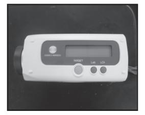
Fig. 1: Colour reader (CR-10, Konica Minolta, Japan)
