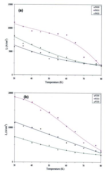
Fig. 1: Critical current density  $J_c vs.$  temperature with different temperature dependences for (a) Bi-2223 tape (b) after  $Co_3O_4$  added
