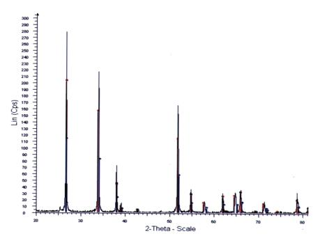
Fig. 3: X-ray diffraction patterns of 5 wt% TiO2-SnO2 catalytic pellet sintered at 650°C for 2 h
