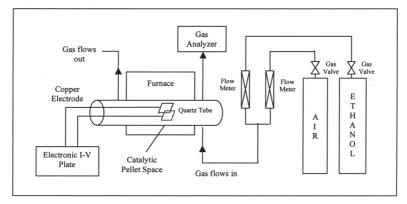
Fig. 1: Experimental rig setup
