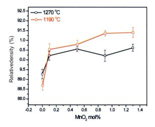
Fig. 2: Variation of density with MnO<sub>2</sub>
