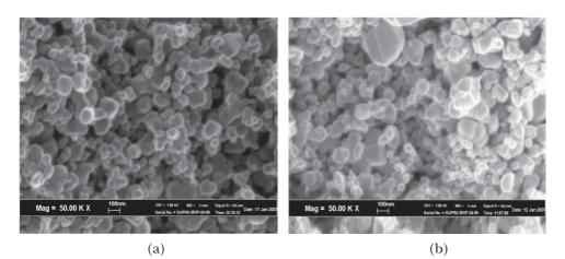
Fig. 2: Surface morphology of catalytic pellet: (a) pure  $SnO_2$ , (b)  $SnO_2$ -5%  $TiO_2$
