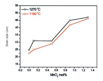
Fig. 3: Variation of grain size with MnO<sub>2</sub>
