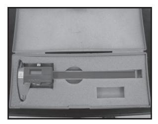
Fig. 3: Digital vernier caliper (500-196-20, Mitutoyo, Japan)
