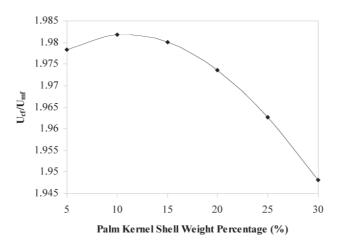
Fig. 6:  $U_{cf}/U_{mf}$  ratio for mixture of silica sand and palm kernel shell
