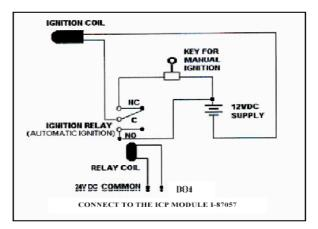
Fig. 1: Schematic diagram output signal of the ignition system
