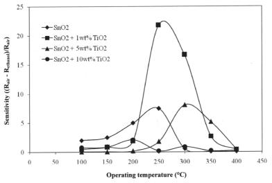
Fig. 5: Sensitivity of ethanol detection at various temperatures
