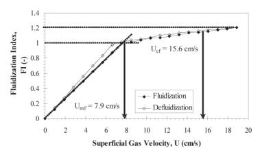
Fig. 5: Fluidization index versus superficial gas velocity for mixture of 85% silica sand and 15% palm kernel shell
