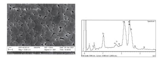
Fig. 5: SEM micrograph for 1.3 mol% and EDX spectrum at the grain boundary for 0.1 mol% MnO, at 1190 °C sintering temperature
