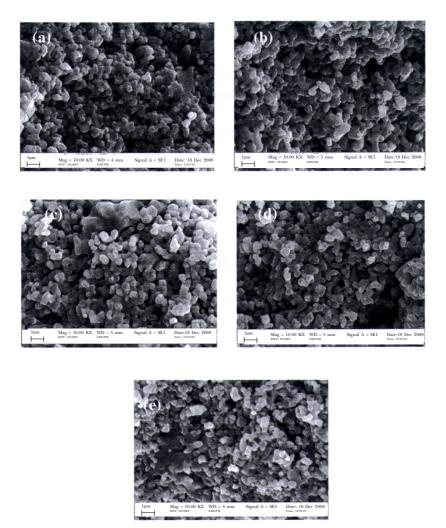
Fig. 7: SEM micrograph of fractured SnO2-CuO samples at different composition (a)10 mol% CuO (b) 20 mol% CuO (c) 30 mol% CuO (d) 40 mol% CuO (e) 50 mol% CuO, at 10,000 magnification
