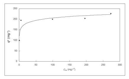
Fig. 2: Adsorption isotherm of methylene blue by CS850A
