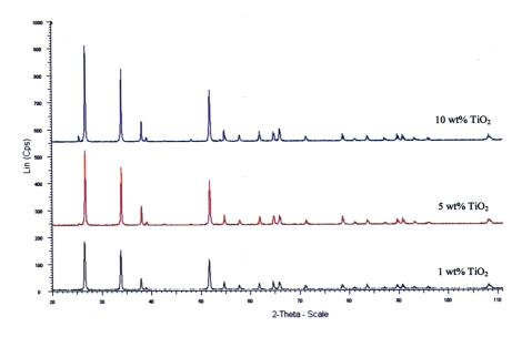
Fig. 4: X-ray diffraction patterns of the catalytic pellet with different TiO, contents sintered at 650°C for 2 h
